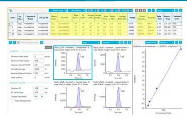
Figure 41. Negative Mode Performance of SCIEX X500R QTOF System for Analysis of Amo/pentobarbital
