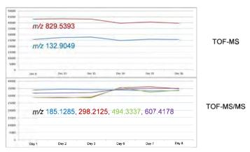
Figure 5. Resolution of the SCIEX X500R QTOF System Over a Week's Period for Selected m/z; both TOF-MS and TOF-MS/MS
