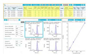
Figure 42. Negative Mode Performance of SCIEX X500R QTOF System for Analysis of THC-COOH
