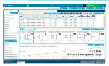
Figure 6. Linearity of the SCIEX X500R QTOF System shown for Asenapine (0.5 ng/mL to 1000 ng/mL)
