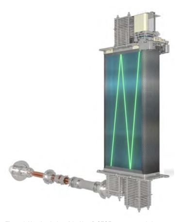
**Figure 1.** N-optics design of the X500R QTOF system to maximize resolution while maintaining benchtop design and a minimized footprint, 6 heater drones are integrated into the TOF path to maintain mass accuracy and robustness
